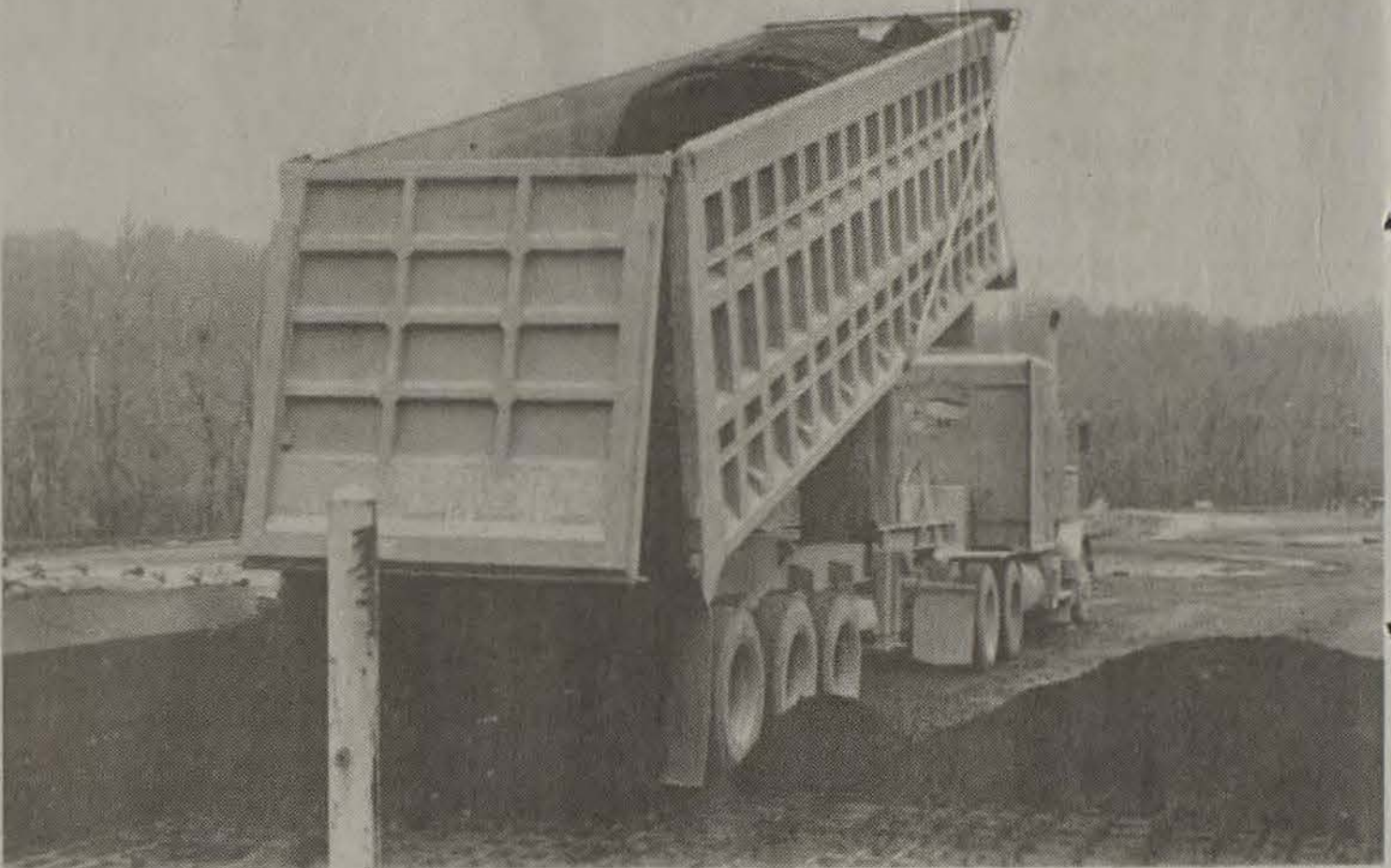
After hauling a load of coal to its destination, the trucks must unload carefully. Flap said unloading can be dangerous because of the possibility the truck may turn over because of the disproportion of the weight. The truck pictured above is unloading the coal in the "hopper" at American Electric Power, near Ashland. (photo by Chris McDavid)
